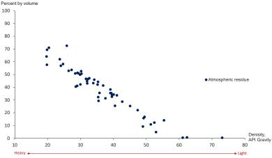
NOTES: Figure plots the amount by volume of atmospheric residue present as a function of API gravity for 54 crude oils. Atmospheric residue and light distillates are the portion of the crude that has a boiling point above 650 or below 330 degrees farenheit, respectively. SOURCE: Exoron's library of rude oil assays.
